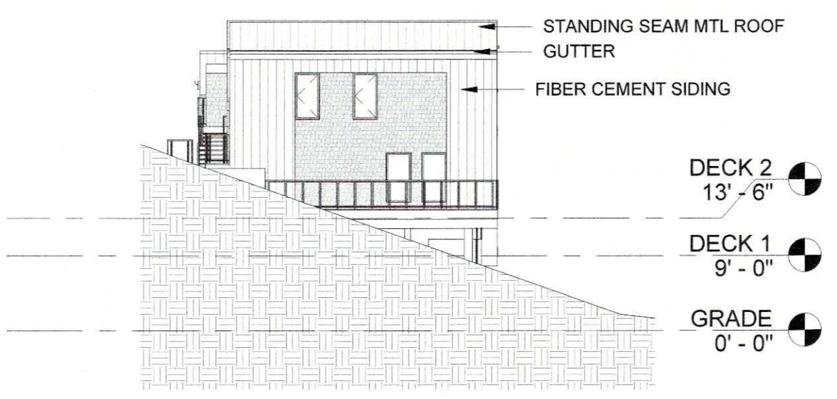
3 NORTH ELEVATION LOOKING SOUTH SCALE | 1/16" = 1'-0"
