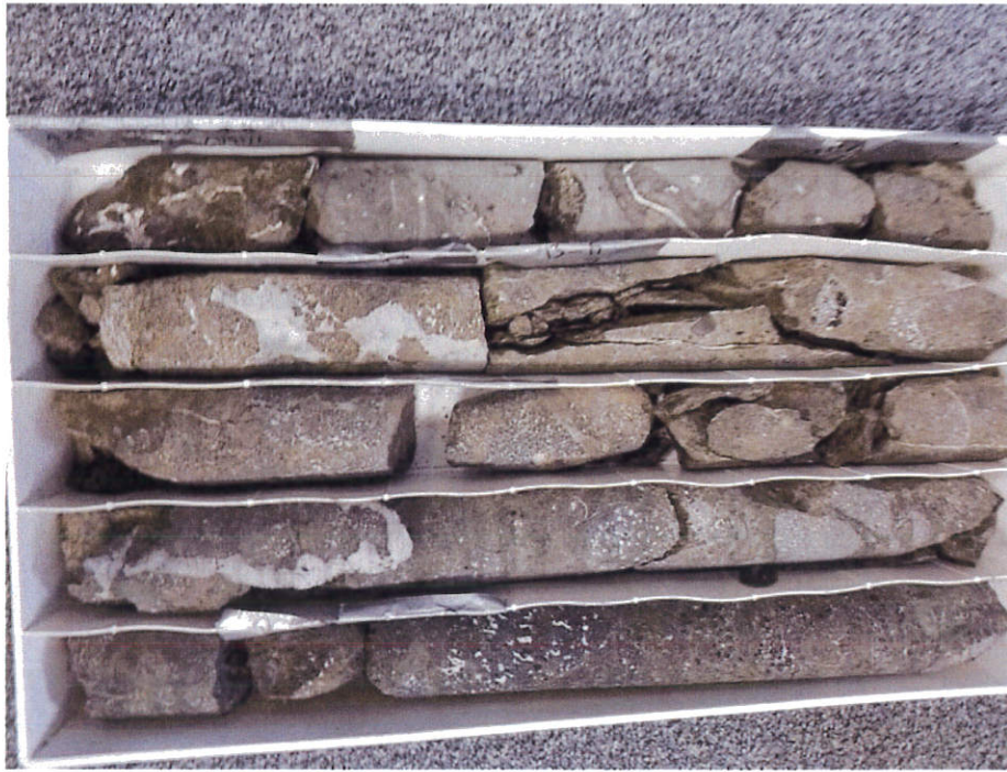
Photo 7 - Close-up view of rock core samples from boring B-2 recovered from approximately 10 to 19.5 feet below ground surface.
