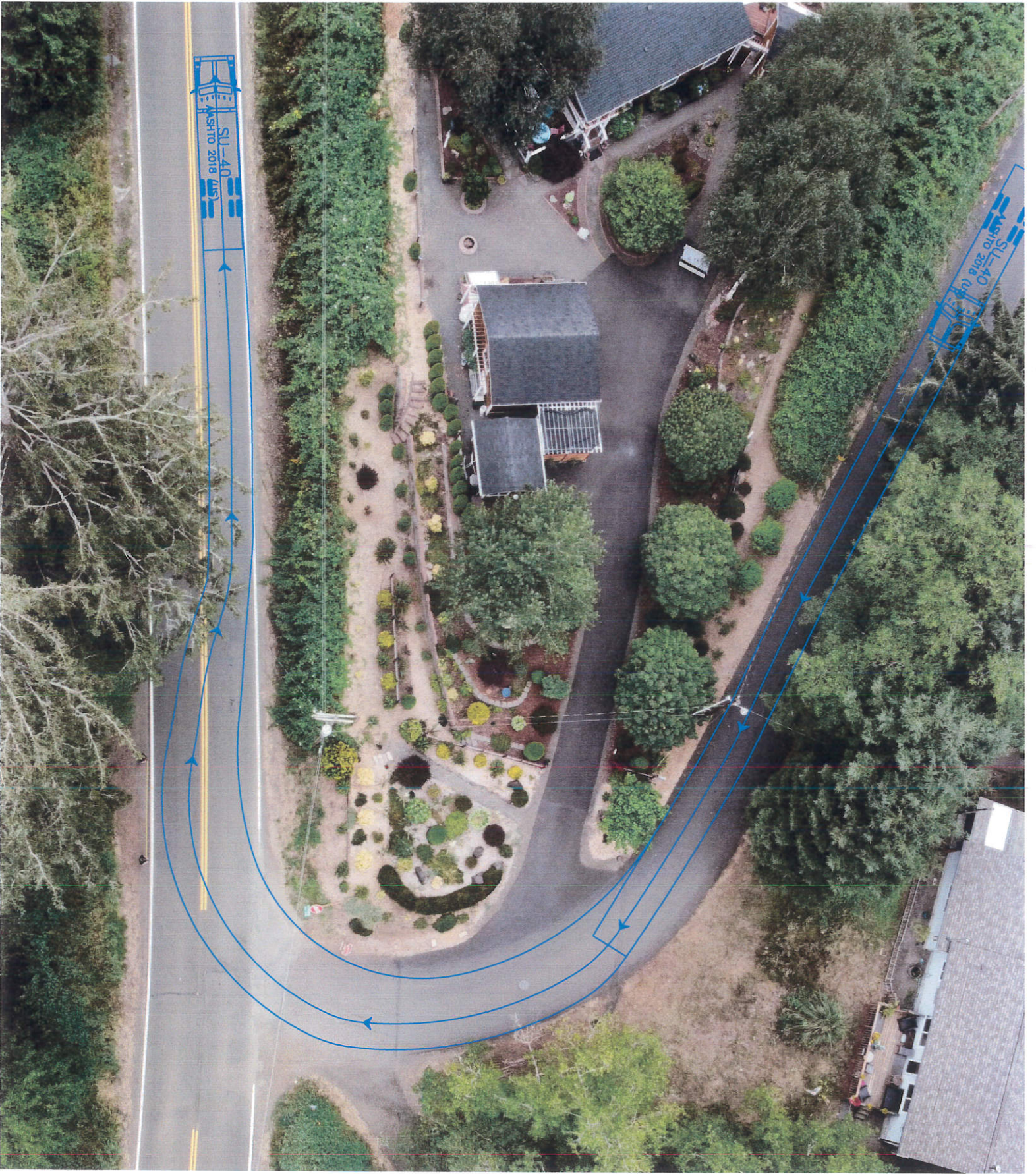
SU-40 Single-Unit Truck Using Both Lanes (Downhill)
