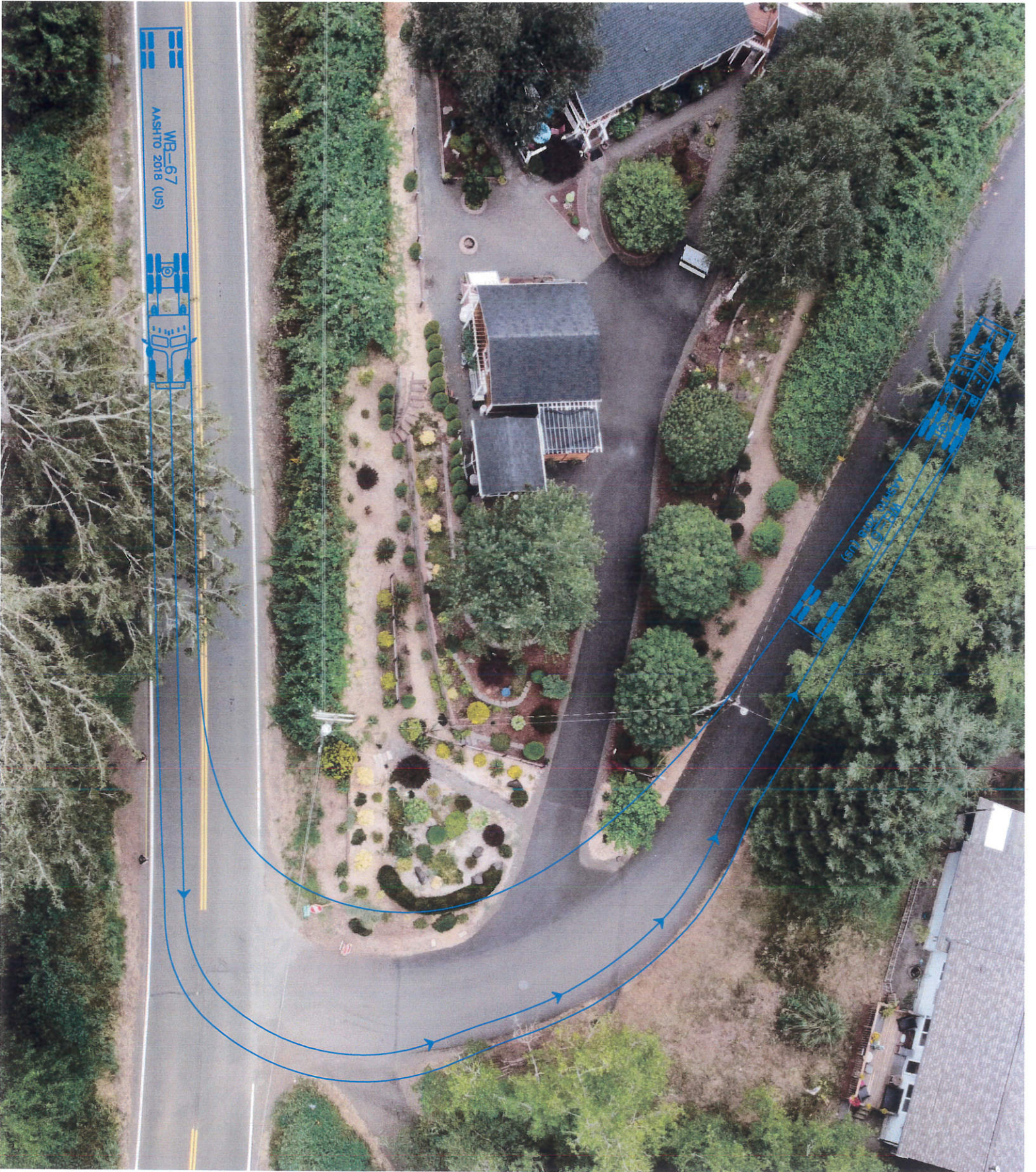
WB-67 Interstate Truck Offtracking (Uphill)
