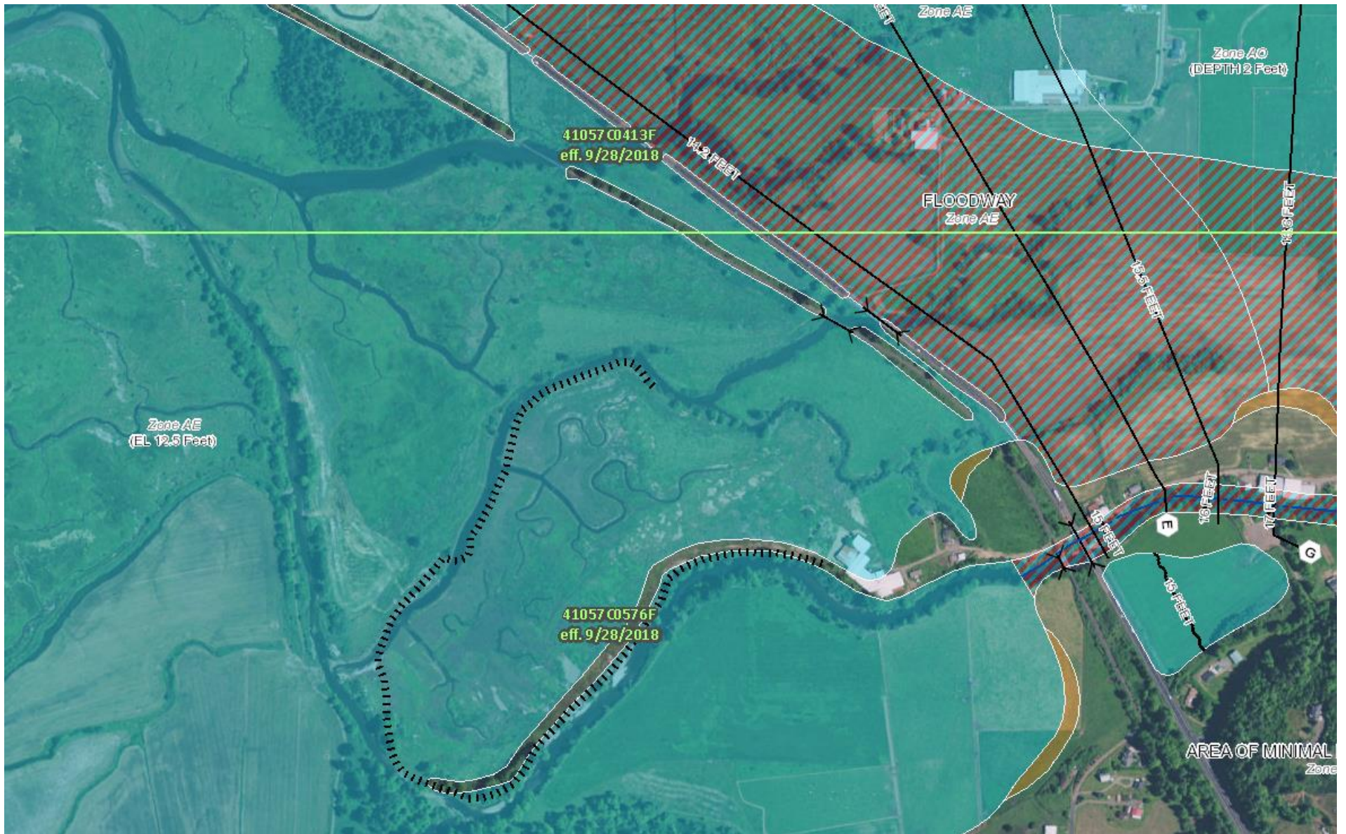
Figure 2. FEMA FIRM Map of Project Area, Kilchis Porter Restoration, Map #41057C0576F, eff. 9/28/2018. Base flood elevation 12.5 feet.
