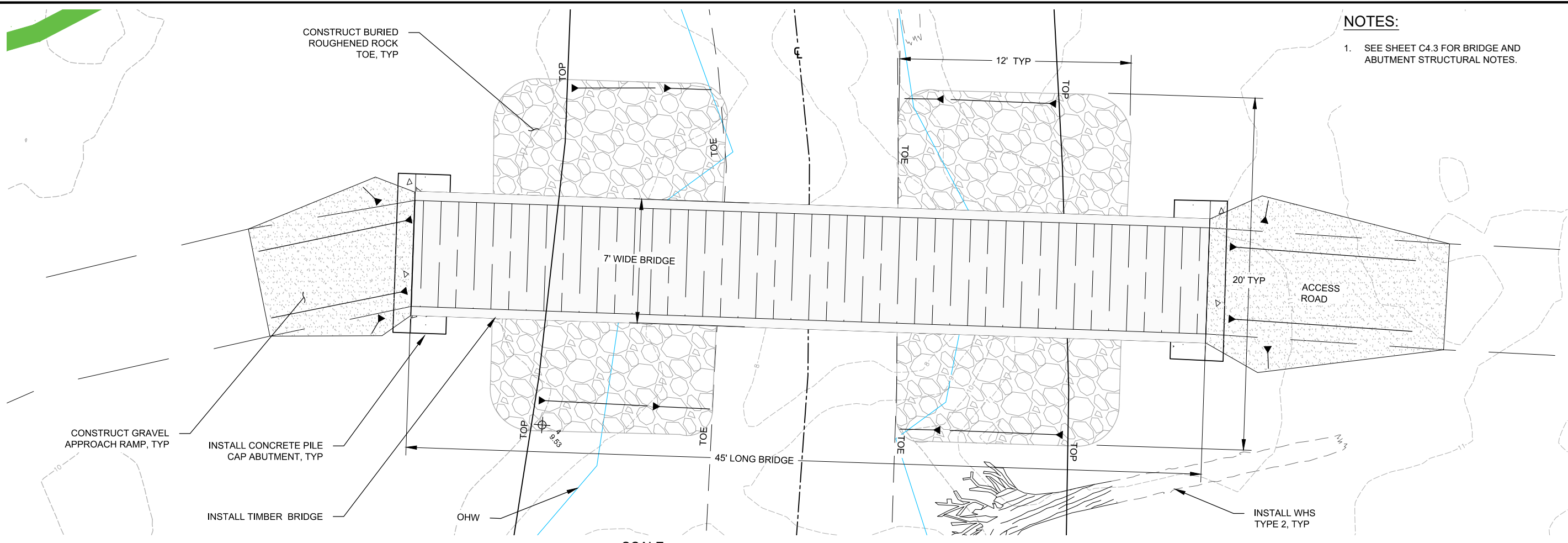
PLAN - PORTER CROSSING TIMBER BRIDGE 1
