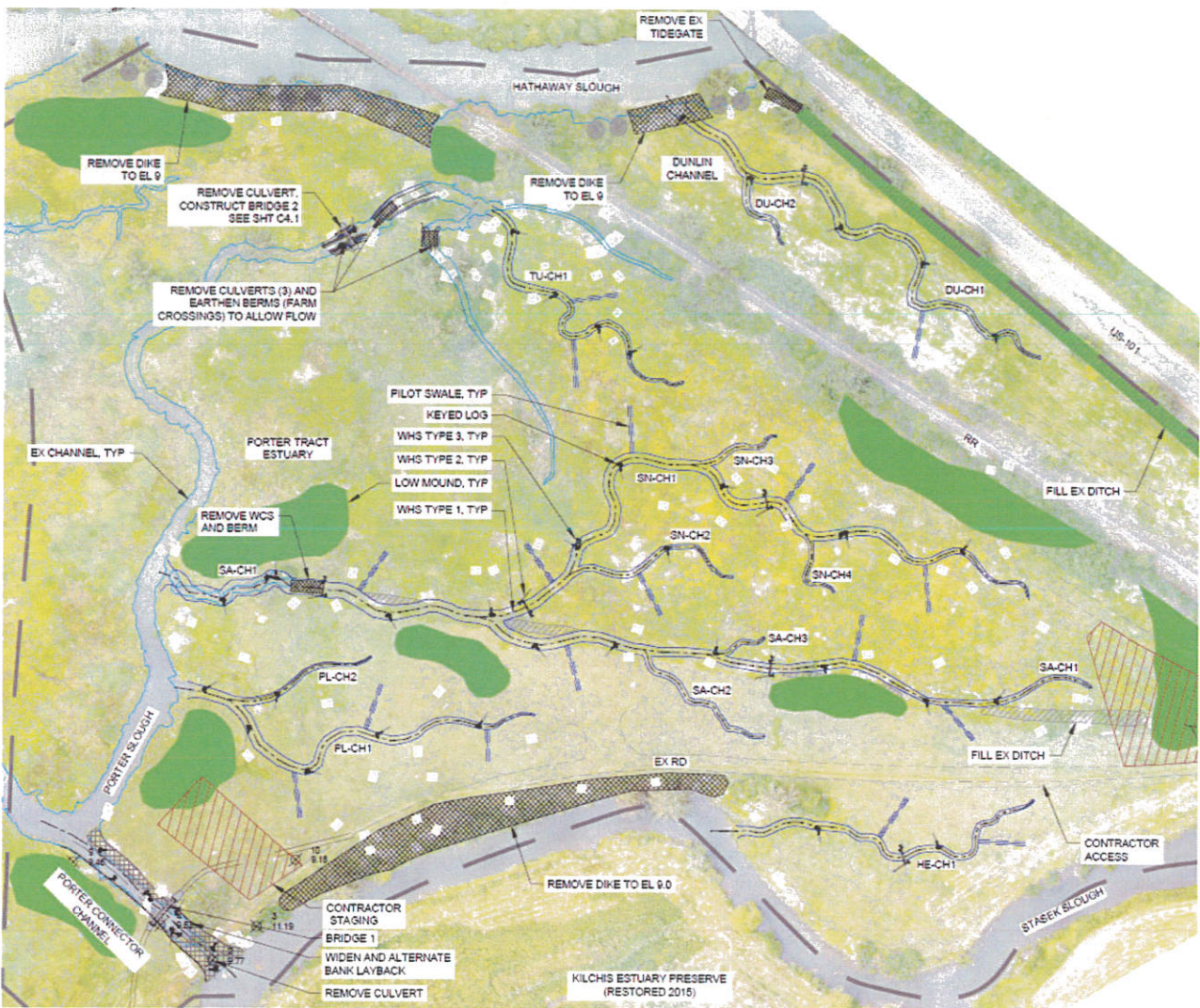
Figure 1 Porter Tract restoration site overview indicating restored channels, filled ditches, dike removals, new bridges, and low mounds.
