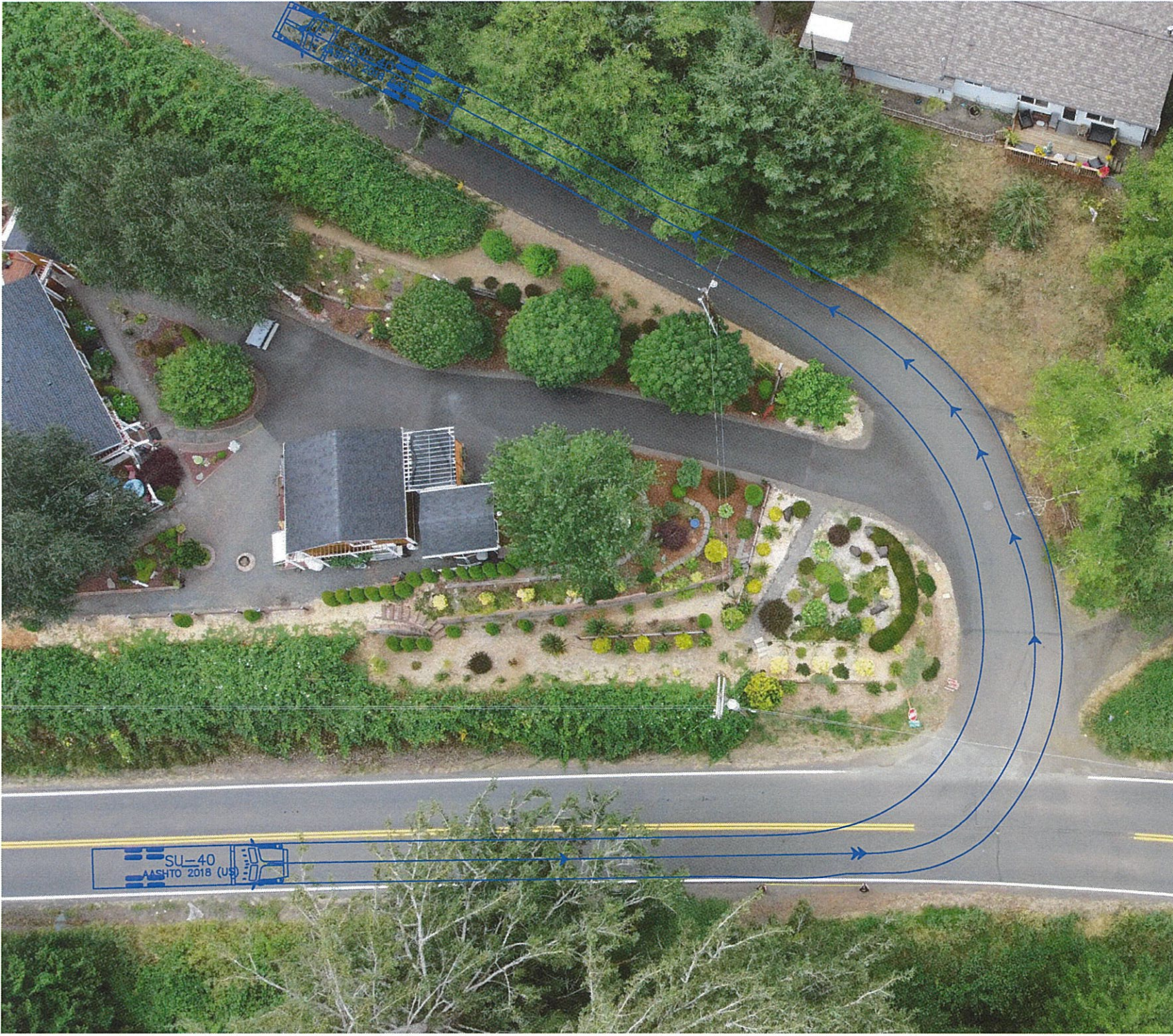
SU-40 Single-Unit Truck Using Both Lanes (Uphill)
