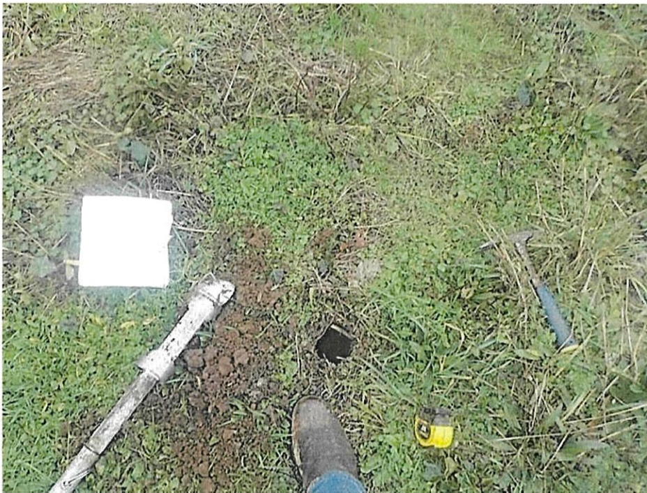
Photo 4 – Close-up view of the silty fill soils encountered in borings B-2 and B-3 on the western portion of the site.
