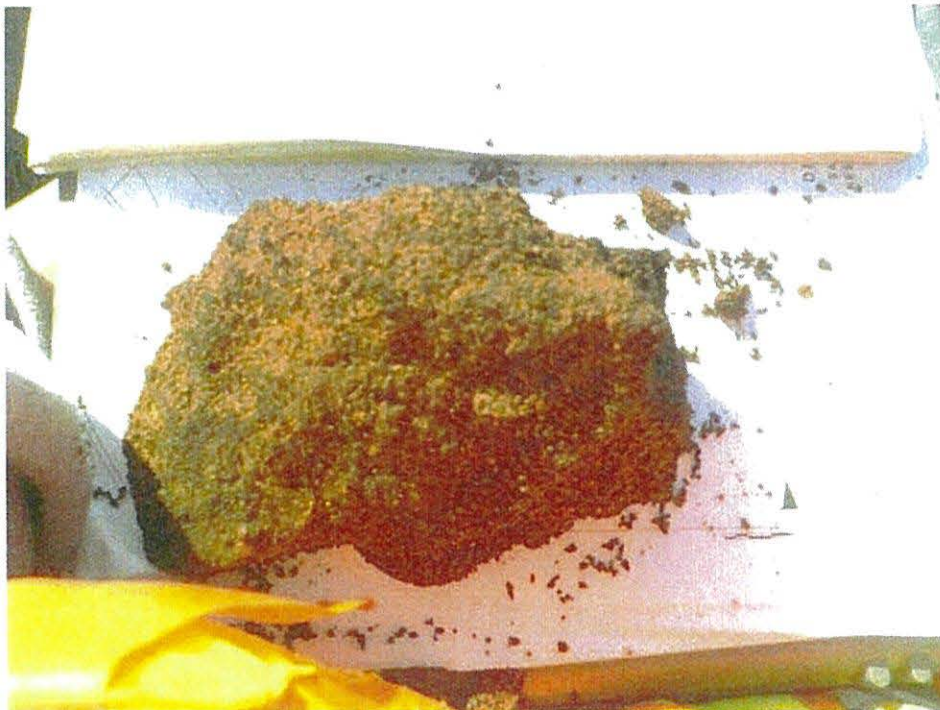
Photo 8 – View of a highly weathered basaltic sandstone fragment typical of those encountered in the test pits (2018).
