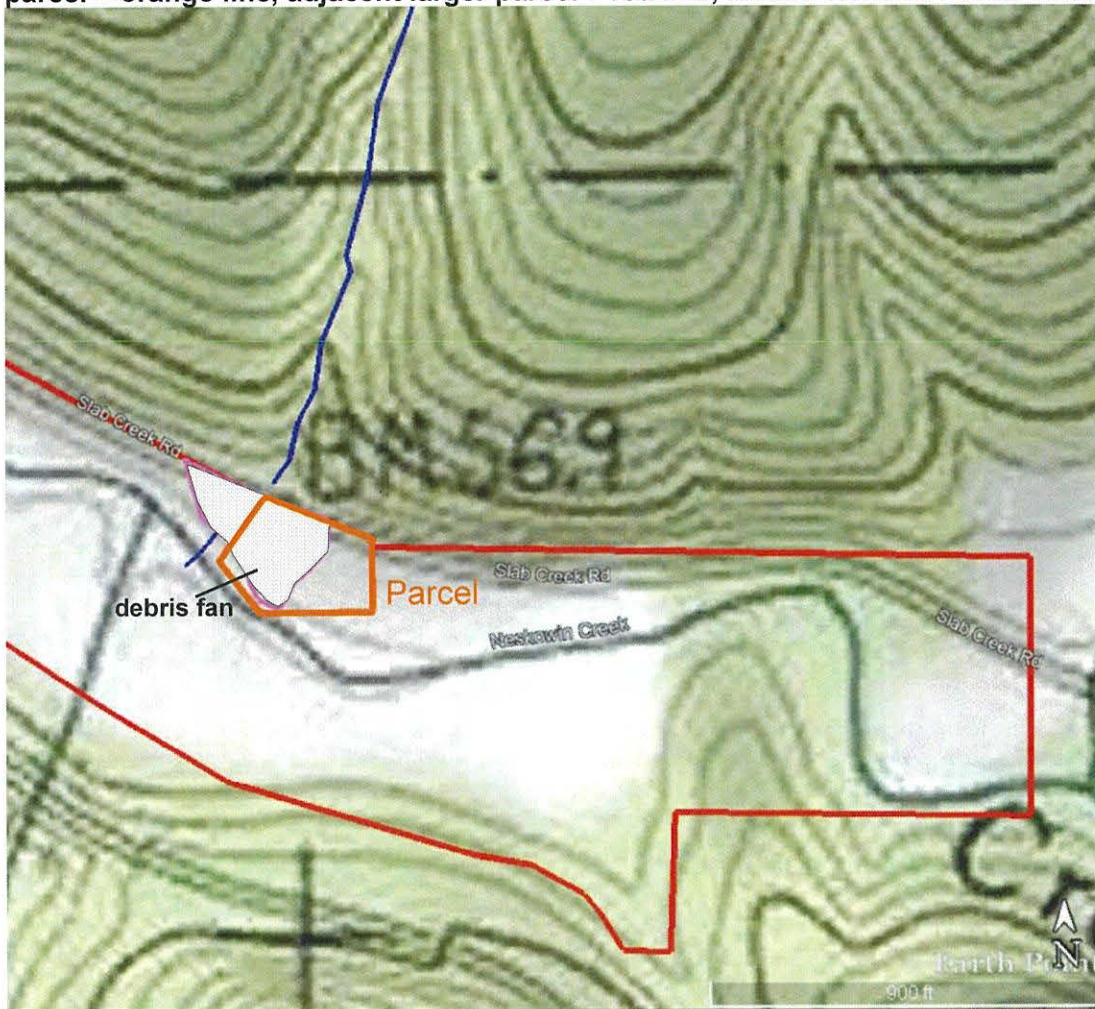
Figure 4. USGS topographic map showing location of debris-fan, parcel = orange line, adjacent larger parcel = red line, stream channel = blue line.
