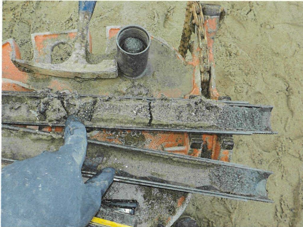
Photo 5 – View of the dense, medium to coarse-grained sand with shell fragments recovered between 30 to 31.5 feet depth in Boring B-1.
