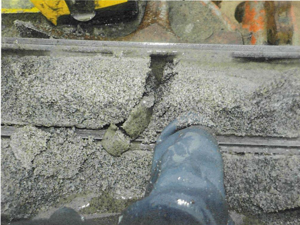
Photo 8 – Close-up view of the very dense, fine-grained, clean sand recovered between 60 to 61.5 feet depth in Boring B-1.
