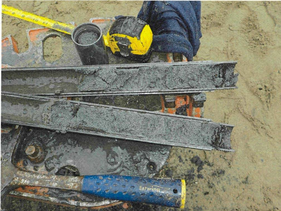
Photo 7 – View of the very dense silty sand with decaying wood fragments recovered between 50 to 51.5 feet depth in Boring B-1.
