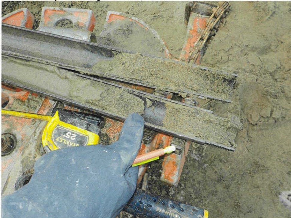
Photo 4 – View of the dense, silty sand recovered between 25 to 26.5 feet depth in Boring B-1.
