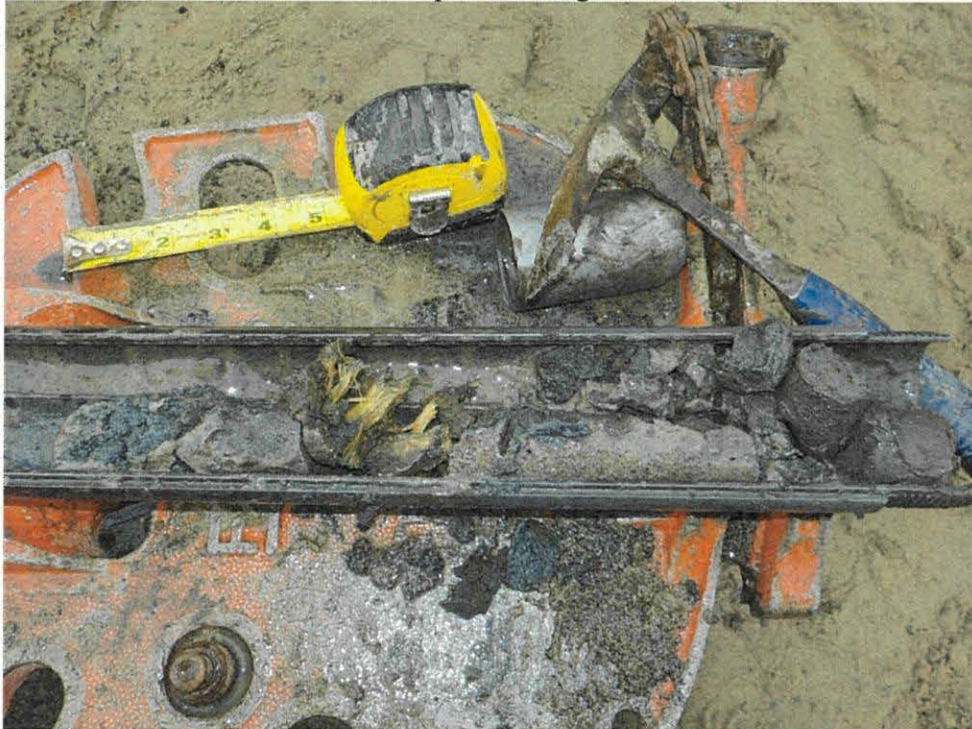
Photo 6 – View of the soft/loose, clayey, silty sand with decaying wood fragments recovered between 37 to 38.5 feet depth in Boring B-1.
