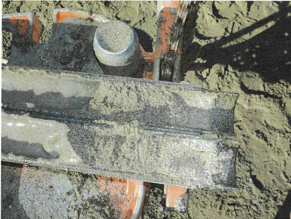
Photo 3 – View of the loose to medium dense, fine-grained sand recovered between 10 to 11.5 feet depth in Boring B-1.
