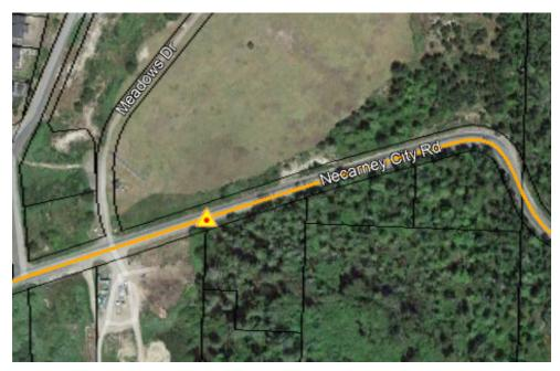
Posted Speed: 35mph, Average Speed: 34.2 mph. 85<sup>th</sup>% Speed: 39.3mph
